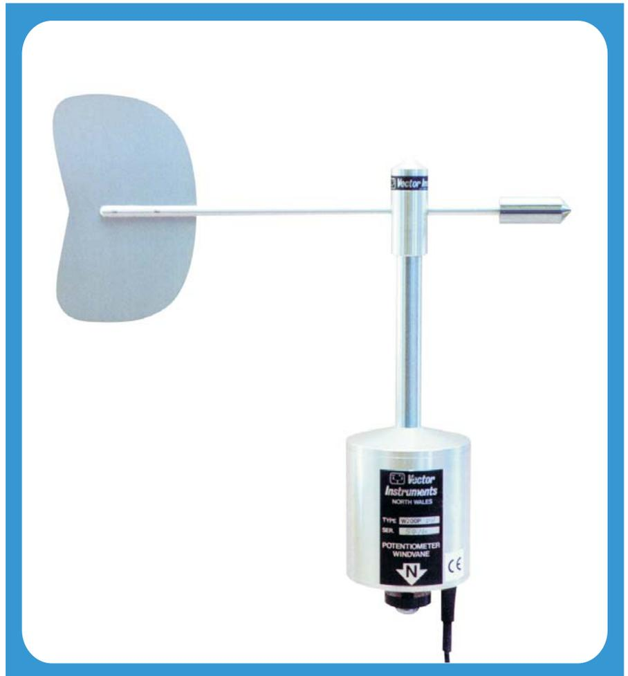
A precision wirewound potentiometer mounted in the same all-weather., corrosion resistant case as the Porton Windvane. The potentiometer has the lowest possible torque consistent with long life and reliable operation. The small gap at North is filled with an insulating material to ensure smooth operation over the full 360°. The vane arm is attached by a unique gravity fastener, giving rapid and reliable attachment and release in portable applications.
