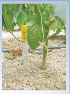
Skye tensiometers have been used as a reference for work in evaluating and developing irrigation management protocols for capacitance sensors. The continuously monitored tensiometers enable periods of under and overirrigation to be readily identified. "Also, because their measurements are not affected by soil salinity, they enable us to identify when changes in soil salinity affect the calibration of the capacitance sensors" added Dr. Thompson.
