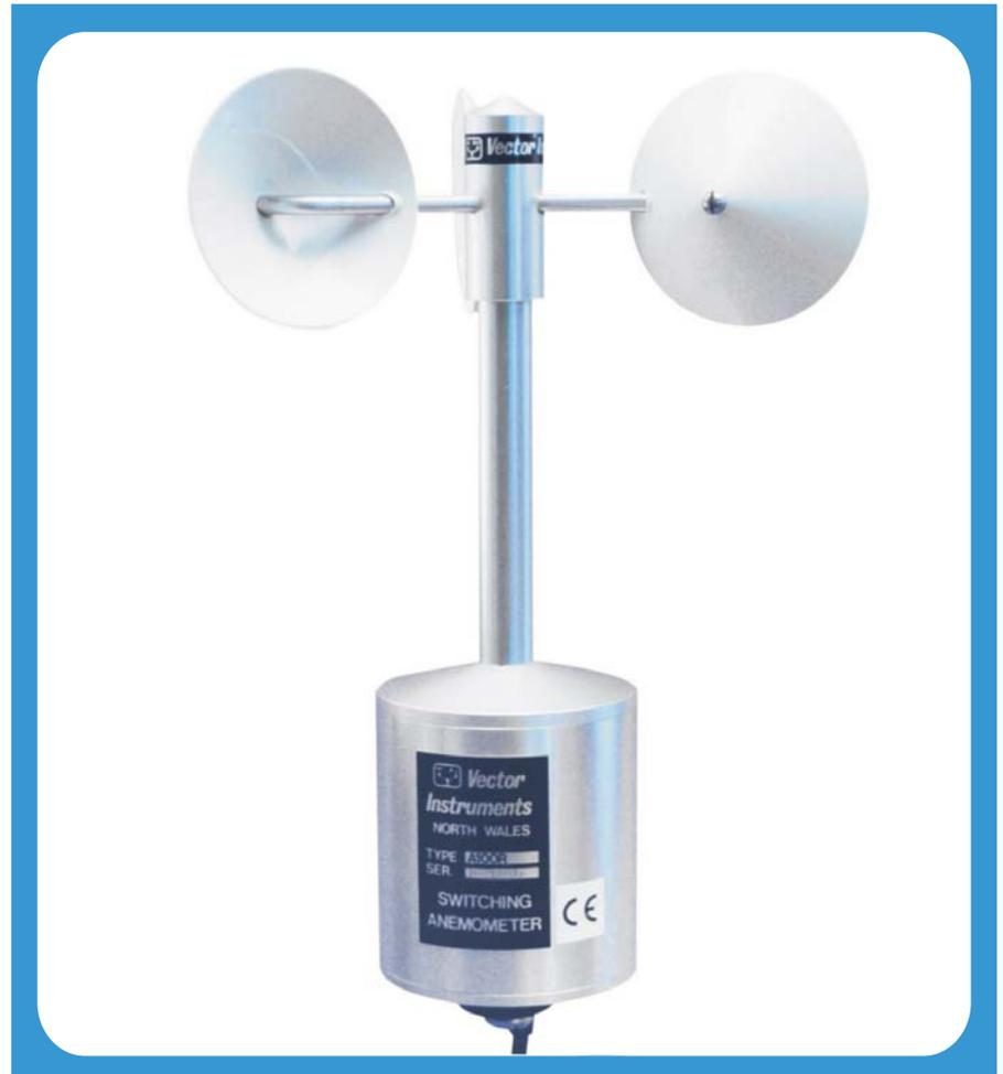
An anemometer for run of wind measurements, or operation with an electronic counter to determine average wind speed. A magnet turns with the rotor spindle and the resulting varying field causes a mercury wetted reed switch to make and break contact once per revolution of the rotor. The contacts are bounce free, simplifying connection to electronic circuits, and no power is required apart from that necessary to detect contact closure, thus
