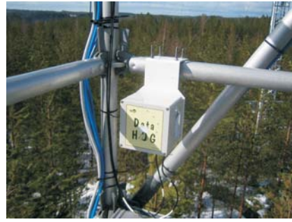
DataHog logger collecting NDVI data
