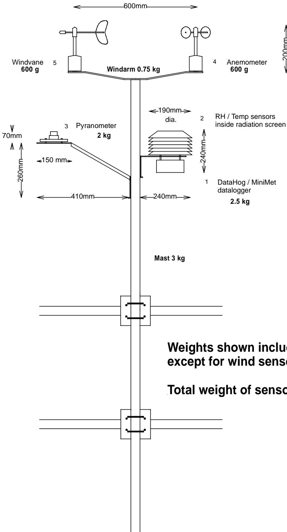
The pole itself is clamped to the horizontal bars of the handrail. If possible the bottom of the pole is also secured by a base plate (supplied). The base plate can be attached to the roof or ground by any appropriate method, e.g. bolts, glue etc.
