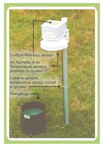
Helios Mini can be programmed to record the weather parameters throughout the day, for example every half hour or hour, not just once or twice a day as is usual with manual stations. This allows the recording of the actual time at which the maximum / minimum temperatures or rainfall occurred.
