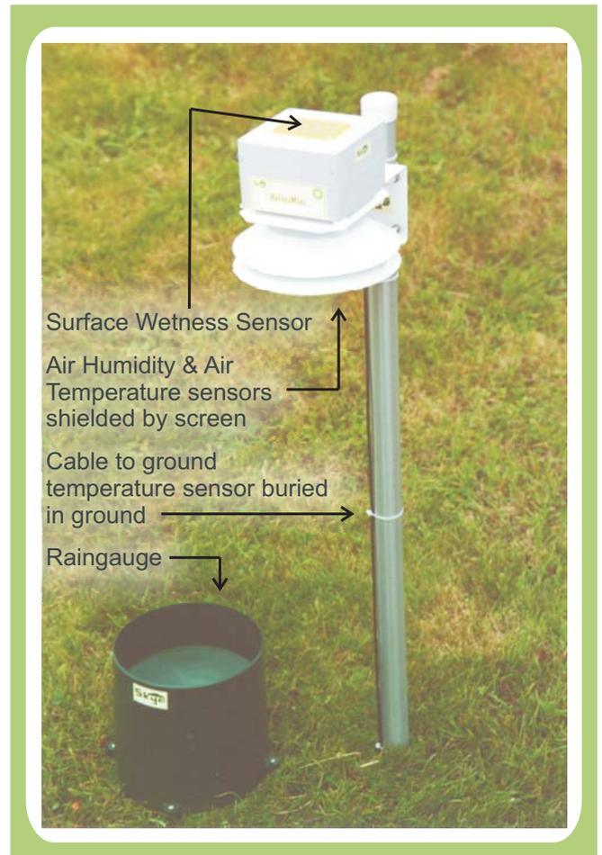
Skye Instruments are well known for the manufacture of high quality automatic weather stations. The Helios Mini is a low cost addition to the range making such automatic measurements available to all.
