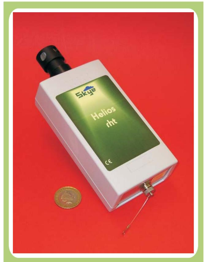
Skye dataloggers, it is only the housing which is more compact. When measuring air temperature it is important to ensure the sensor tip is not located in direct sunlight or near other sources of light or heat, to ensure true temperature recordings.
