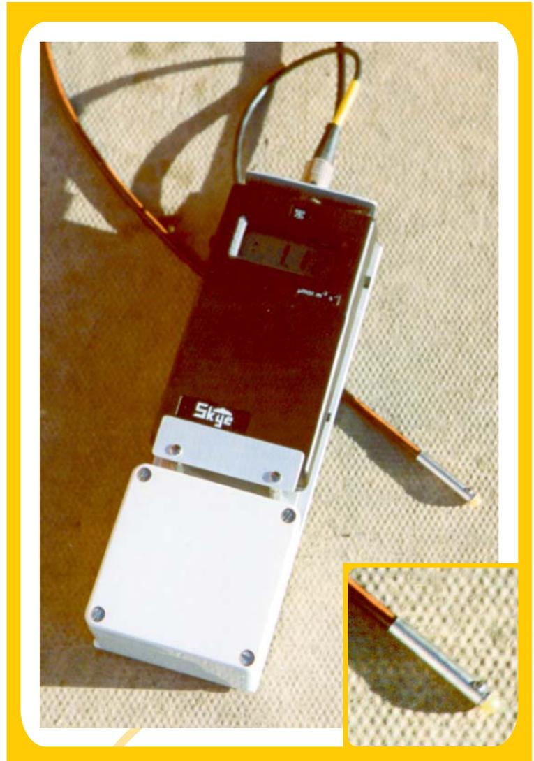
This hand-held system measures light within the same ranges and responses as other Skye sensors, except that the light is collected at the end of a long fibre optic probe extension. Choose from any of the standard Skye sensors (excluding UV and UVB), or your own preferred response between 400 - 800 nm. 1 or 2
