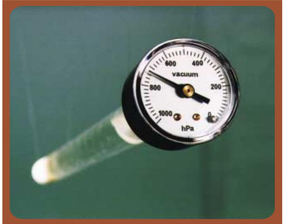
The Dial Tensiometer is a low cost version of Skye's successful field tensiometer range. Tensiometers measure the water availability to plant roots, and so can be used in irrigation scheduling and crop management.
