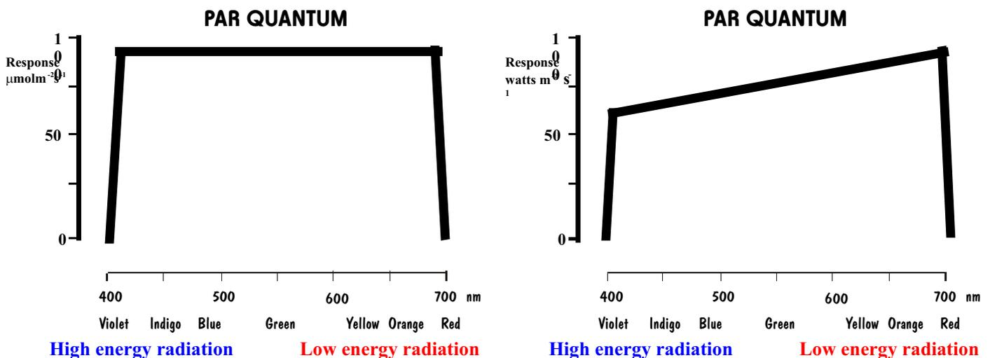
The PAR Energy sensor is designed to have a flat square response when plotted in an energy curve.
