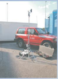
The data can be seen in real time and can be collected via RS232 and/or an optional GSM connection.
