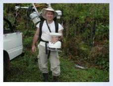
Dr Scott Henderson of Oxford University is recording microclimatic variables under the canopy of an invasive tree species that may be responsible for plant community composition differences. He is using the DataHog with Skye sensors to monitor RH, air and soil temperature, rainfall and PAR radiation simultaneously both under the tree canopy and about 10m away in an open area of native vegetation outside the tree's influence.
